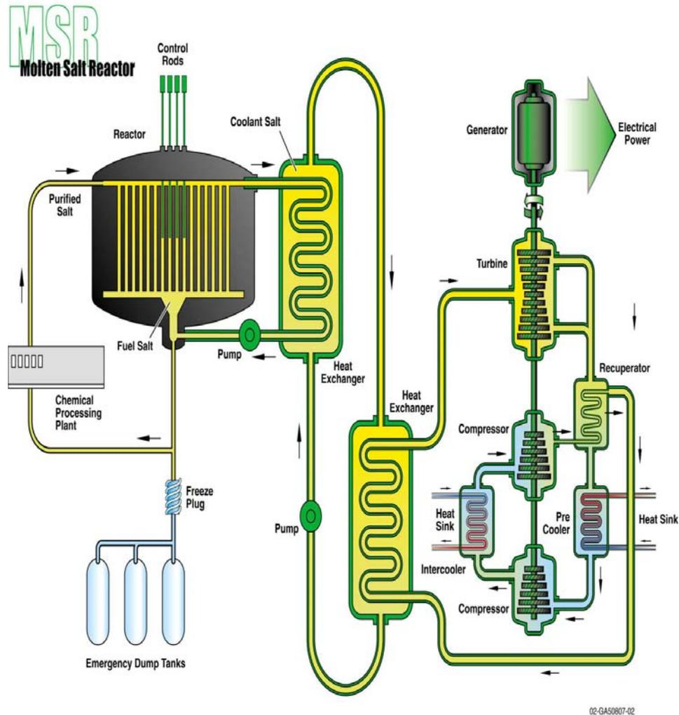
Figure A6.1. MSR with Brayton power cycle.
